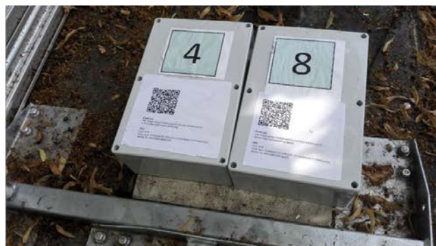
Figure 21. Deployment of Raptor nodes O3 and NO2 with QR code
