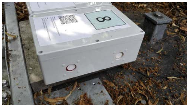
Figure 21. Deployment of Raptor nodes O3 and NO2 with QR code
