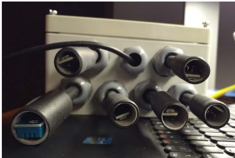
Figure 8. Insert sensors in sensor tubes
