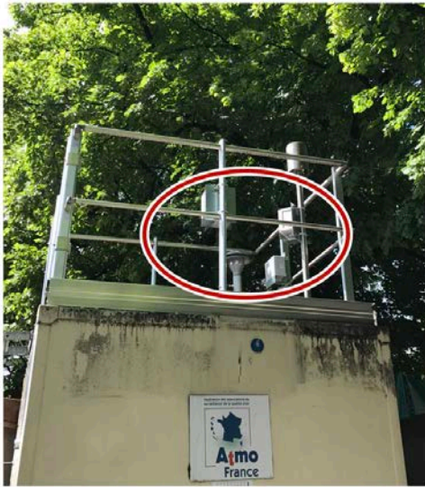
Figure 18. End-device deployed on the roof of ATMO Auvergne reference station in Clermont-Ferrand.
