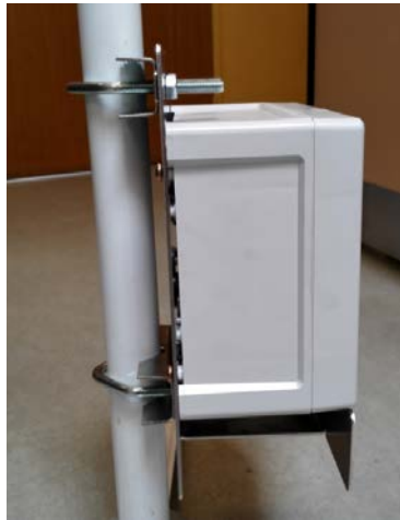
Figure 10. New packaging of RAPTORG2 End-device for outdoor deployment
