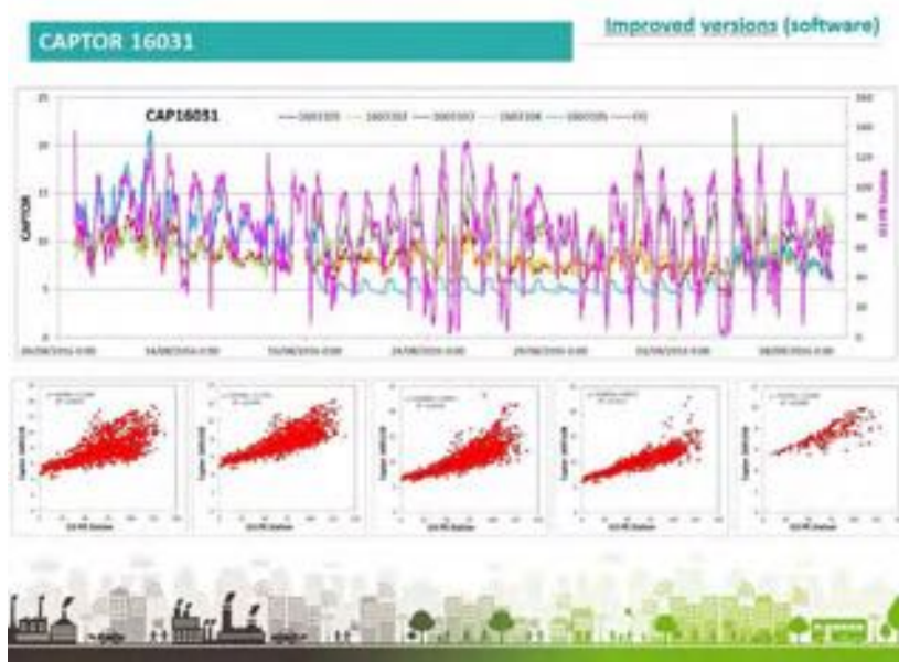
Figure 4. Inter-comparison between sensor and reference data for one node including the improvements and lessons learnt from the 2016 summer campaign.
