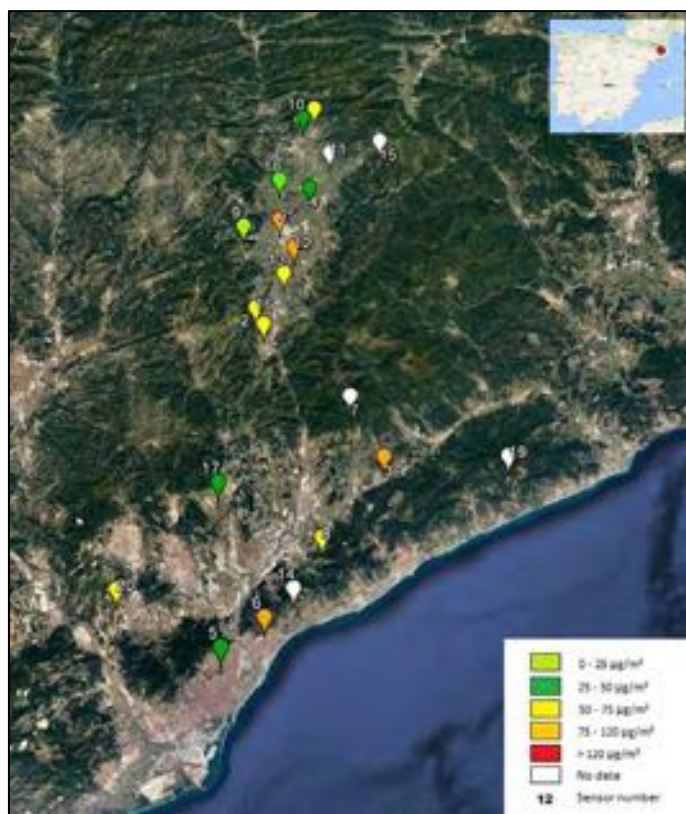
Figure 8. Spatial distribution of mean hourly ozone concentrations monitored with Captor nodes during the 2016 summer campaign.
