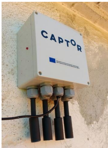
CAPTOR: metal oxide low-cost sensors (UPC)
